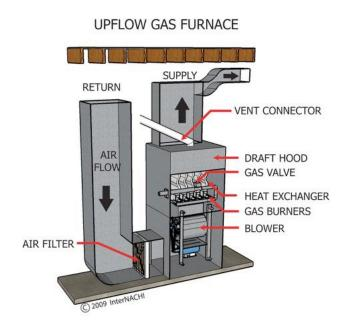
Most furnaces that can qualify for the ENERGY STAR will be "condensing" furnaces where the transfer of heat is so thorough water or condensate is a byproduct of combustion. This condensing occurs with systems over 90 percent efficient. Another feature of efficient furnaces is a highly efficient blower motor (commonly an ECM, Electronically Commutated Motor, or another type of "advanced main air circulating fan").
